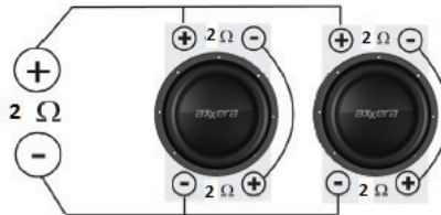
(2) 2 ohm DVC Speaker = 2 ohm Load
