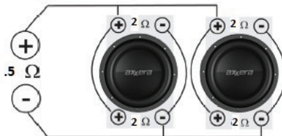
(2) 2ohm DVC Speaker = .5 ohm Load
