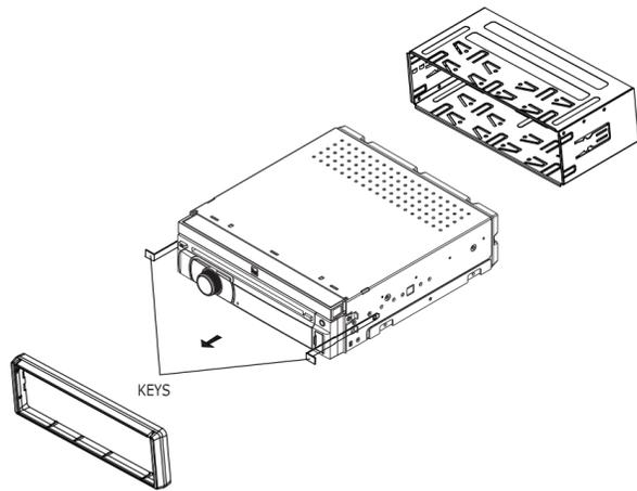
TYPICAL FRONT-LOAD DIN MOUNTING METHOD
