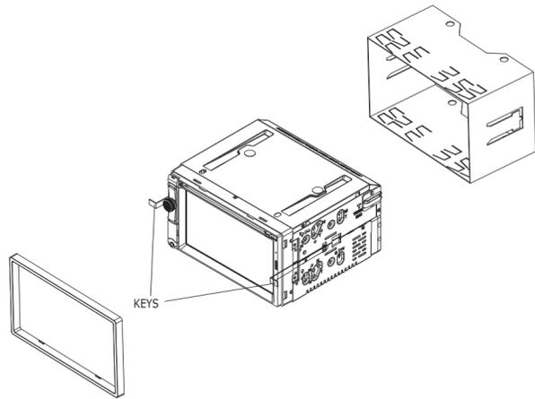
TYPICAL FRONT-LOAD DIN MOUNTING METHOD
